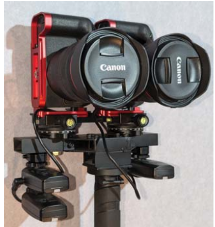
Twin Canon RP cameras with superzoom lenses (above) and wide angle lenses (right)
